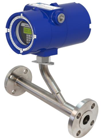
Inline thermal mass flow meters provide a plug-and-play solution for many applications, while providing a cost-effective solution for high accuracy and no maintenance. Flow sensitivity is increased because the sensors are placed directly in the flow stream without the protection needed with insertion meters. There are 10 models available in pipe diameters ranging from 3/8" to 4". The Kurz power-limiting design and constant temperature sensor control prevents sensor overheat at zero flow.
